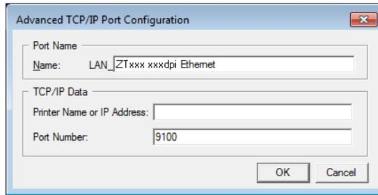
19. Enter the printer's IP address. This could be one that was assigned automatically or one that you specified manually in the previous section.
