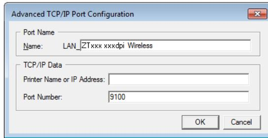
14. Enter the printer's IP address. This could be one that was assigned automatically or one that you specified manually in the previous section.
