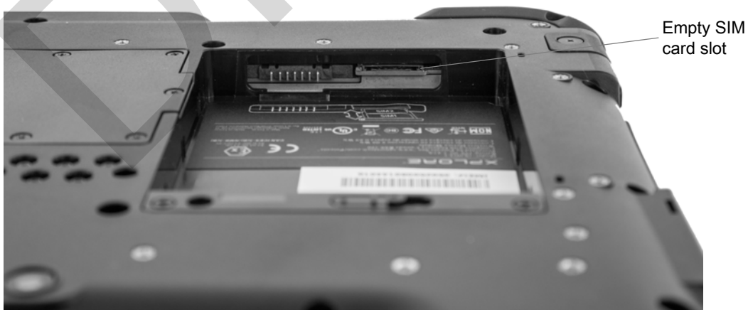
Figure 1 Empty SIM Card Slot
