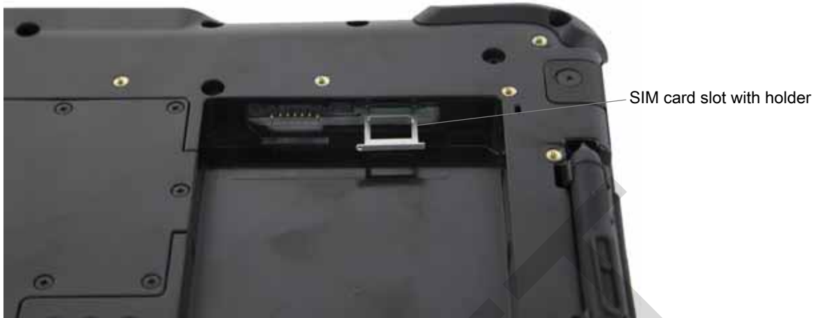
Figure 2 SIM Card Slot with Holder
