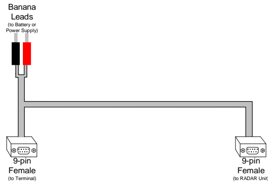
Figure 1 - Communication / Power Cable
