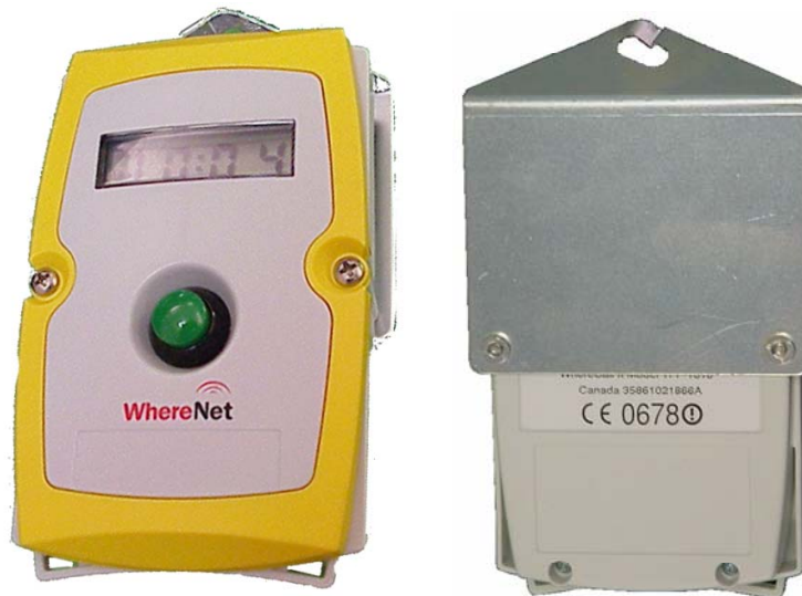
Figure 7: Front & rear view hanging bracket installed
