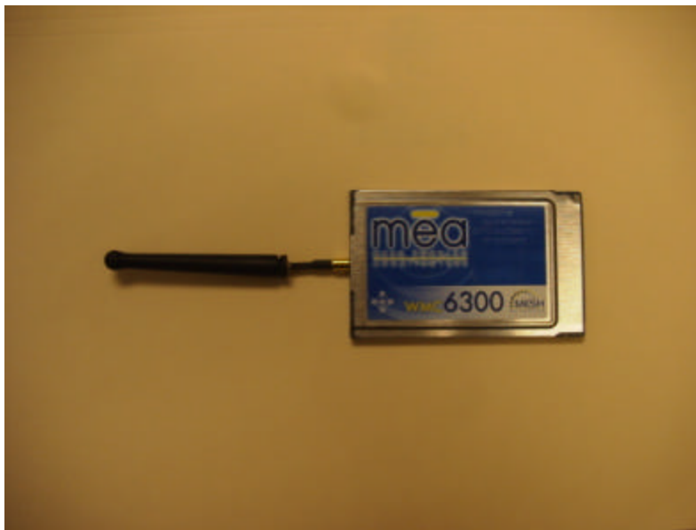
Figure 10. Attach Antenna to the WMC6300
