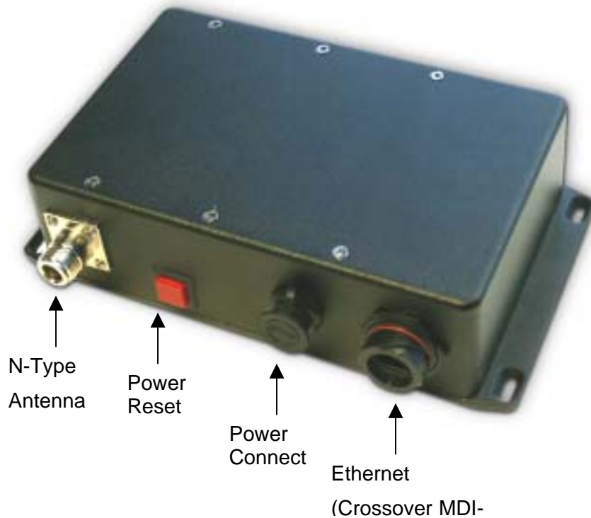
Figure 2-2. PWR External Connection Point
