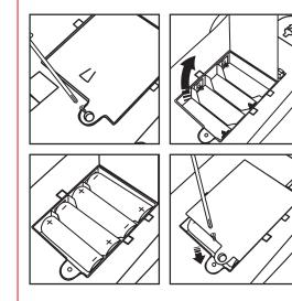
To install batteries into the Wireless RC Car, unscrew the screw on the battery box cover to open the cover. Insert 4 x "AA" 1.5V batteries (Not Included) into the battery box. Batteries should be placed as shown on the diagram.
