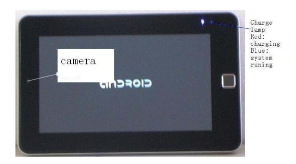
insert an external charger, then charge lamp will turn on; When charge is completed, charge lamp will light turn off
