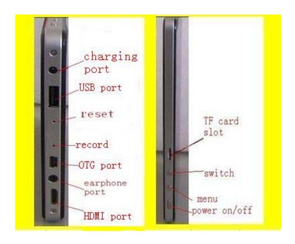
Note: if system halted, please insert one slender material into the reset key ,then system will shutdown
