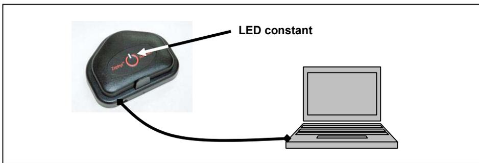
When the LED is illuminated, the battery is charging.
