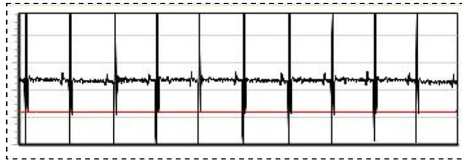
Fig 4.1.1 A good low-noise ECG signal from a static subject with a dry garment
