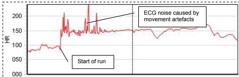
Fig 4.1.2 The subject has started a 3km run with a dry garment. The clean heart rate signal prior to the run is immediately noisy due to movement artefacts generated by the running action, and EMG noise. As the subject's skin moistens with perspiration, the noise clears.
