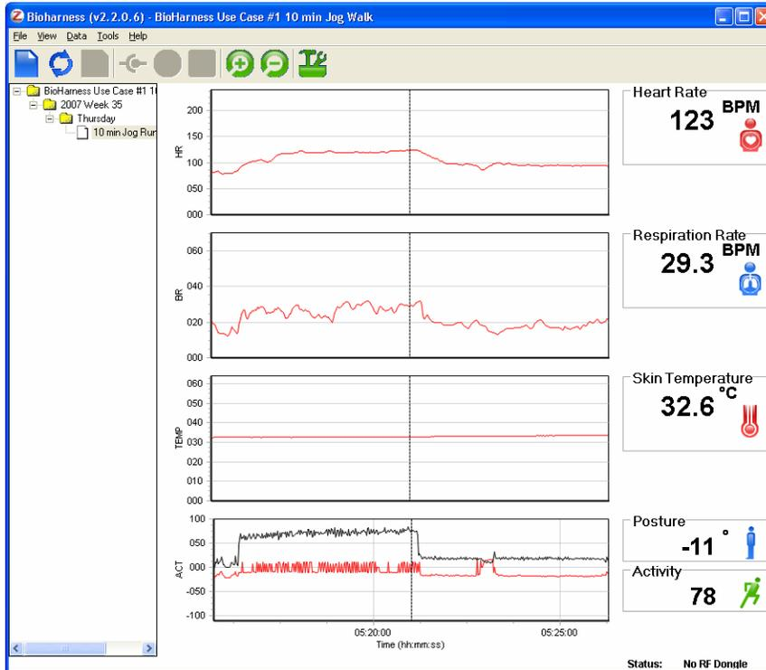
This project has been made in RF recording mode. Raw ECG data is available for export to a csv file. The ECG Raw data and Processed Breathing Waveform have been removed using Graph Settings so as not to obscure the trend data.
