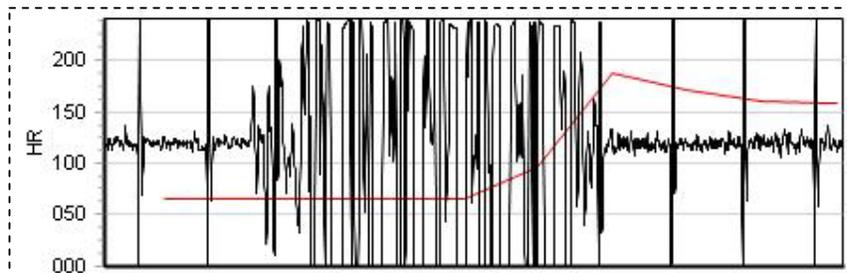
Fig 4.1.3 EMG noise/movement artefacts generated by vigorous arm movement
