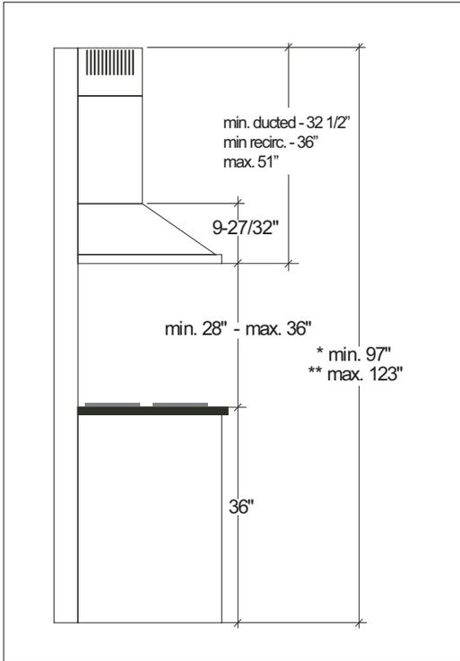
Minimum mount height between range top to hood bottom should be no less than 28".
