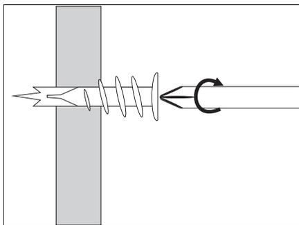
Tap EZ anchor tip into marked drywall locations, turn with screwdriver until seated flush.
