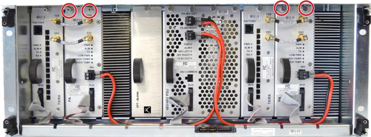
FIGURE 13: Power Amplifier Subrack Locations
