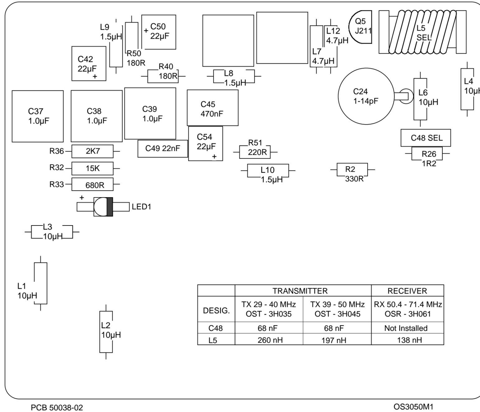
4.1.2 OS(R/T)-3H 29 - 71.4 MHz Analog Board Component Layout (Top)
