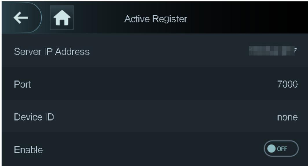
**Step 2** Turn on the automatic registration function and set the parameters.
