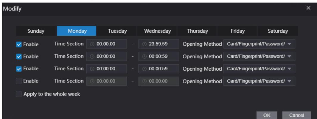
2. Configure the time and the opening method for a time section. You can configure up to four time sections for a single day.
