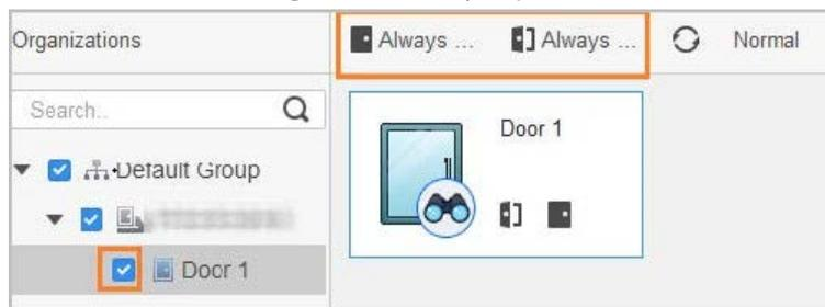
The door will remain open or closed all the time. You can click **Normal** to restore the access control to normal status, and then the door will be open or closed based on the configured verification methods.
