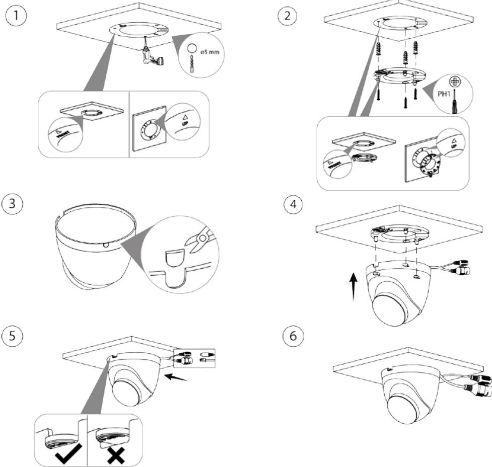
Figure 4-6 Cable going through the mounting surface
