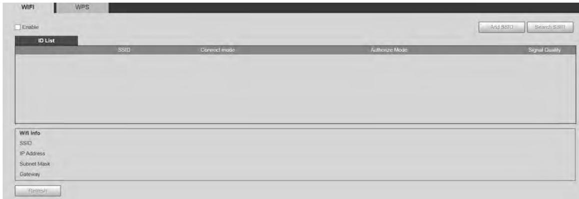
**Step 2** Click **Search SSID**, and Wi-Fi hotspots in the environment of current network camera are displayed.
