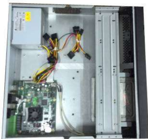
⑦ Put the bracket back. Please adjust the CD-ROM to the proper position so that the button of the front panel is directly facing the pop-up button of the CD-ROM.
