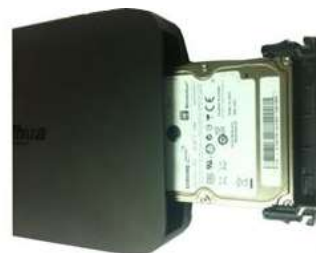
③ Put the HDD into the device
