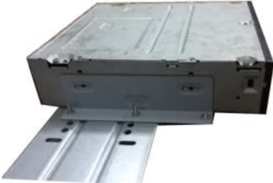
③ Fix the CD-ROM bracket at the HDD bracket.
