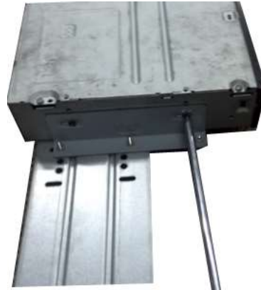
⑥ User screwdriver to fix the screws.
