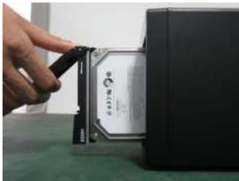
② Put the HDD to the HDD box at the front.
