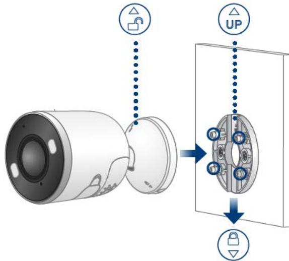
7. Attach the camera to the mounting bracket using the threaded insert at the rear of the camera. Rotate the camera clockwise until attached, then tighten into place with the adjustable nut.
