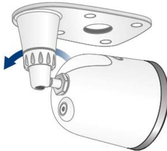
7. Place the bracket over the drilled holes. Using a screwdriver and the provided screws, secure the bracket to the surface.
