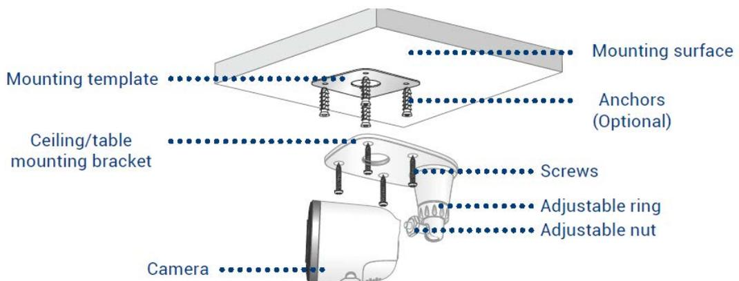
1. Place the mounting template onto the desired location.
