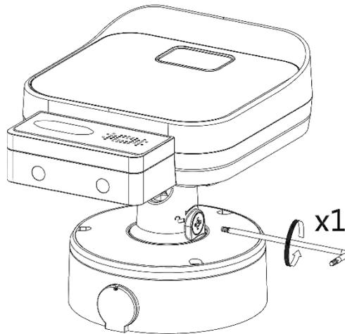
Figure 2-7 Unscrew and remove the junction box
