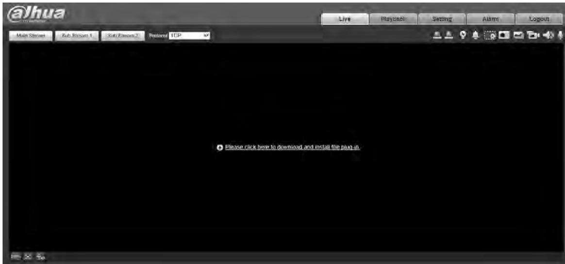
**Step 3** After the plug-in is installed, the login interface is refreshed automatically. Enter username and password again, and then click **Login**. The live view interface is displayed.
