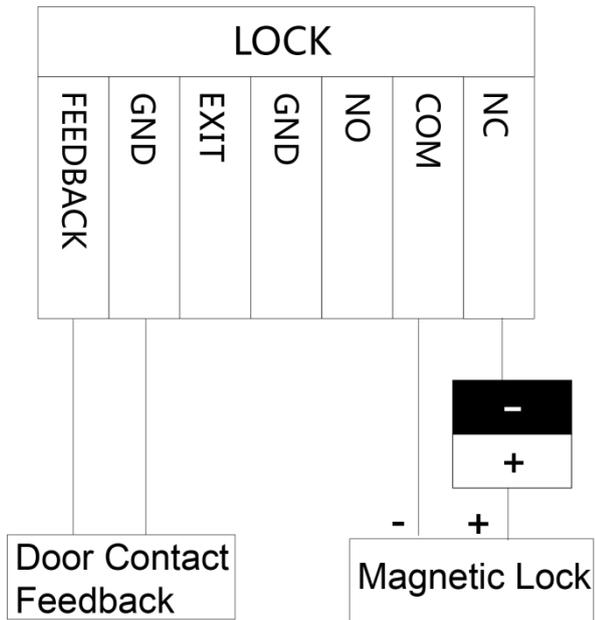
Figure 2-4 Electro-mechanical lock connection
