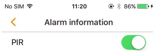
The PIR detection is enabled by default, and the switch shows
