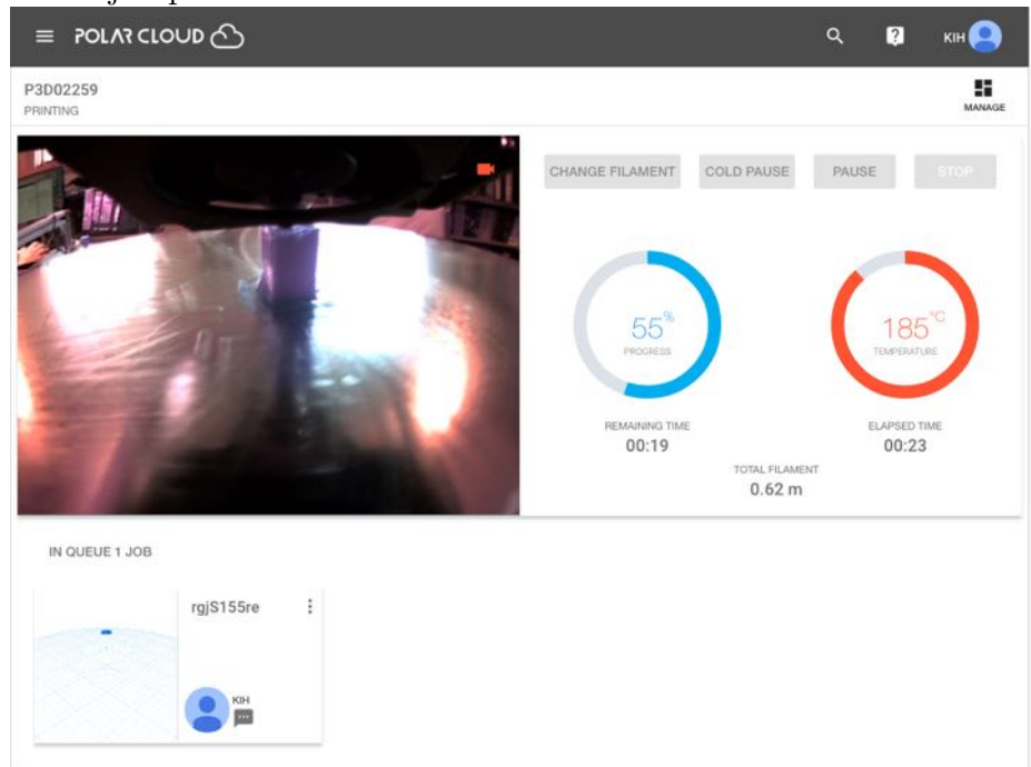
Figure 4.88: Printer dashboard: a member queued job waiting while another member's job prints
