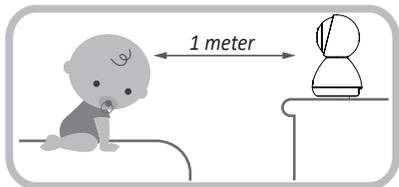
Never place the baby unit or the cord within 1 meter of the crib.
