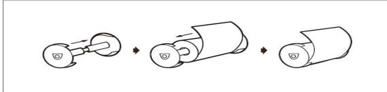
2. Take out the adjustable plate. Open the adjustable plate slightly, install the paper roll in the plate and close it.
