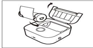
3. Place the paper roll into the printer and straightened the paper as shown in the picture above.
