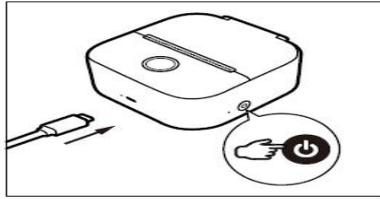
1. Fully charge the battery before using the first time. To turn on the machine, press and hold the power button for 3 seconds.
