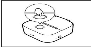
1. Replace the paper by pushing the switch on the printer to open the cover.
