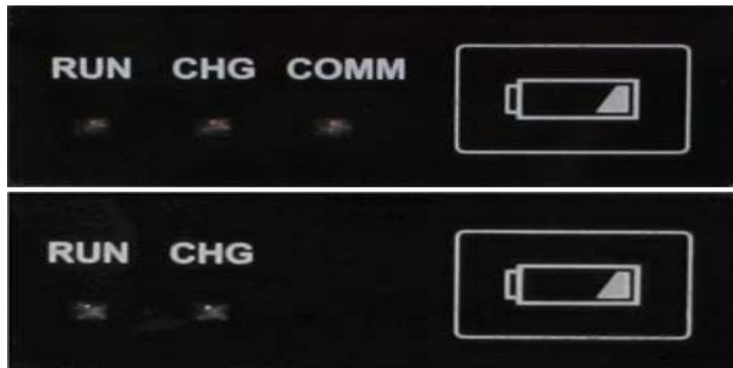
(1) Power Indicator Lamp: When power is normal, the green light is normally on.
