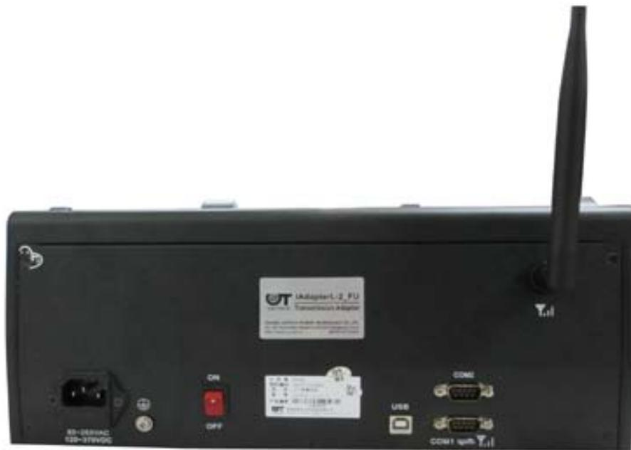
Install the antenna into the antenna input port as blow figure. Turn the antenna to the vertically upward direction.
