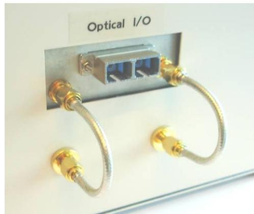
Figure 3-23: Connecting the RF jumper leads on the 277X AU.
