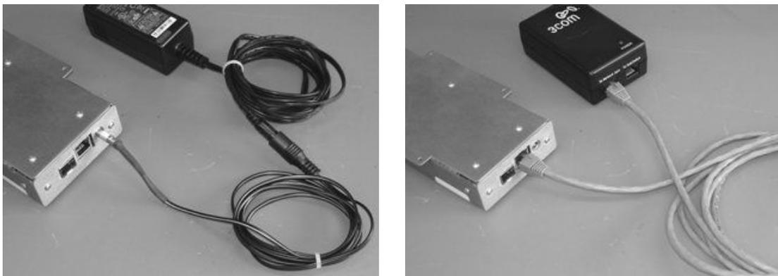
Figure 3-20: Connecting the DC supply unit or the PoE mains adaptor.
