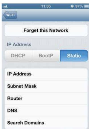
Go to **Settings - Wireless - Selected SSID - advanced settings**, then click on **Static** to enter IP address such as **10.10.10.XXX**. (XXX can be set from 1-128) and Subnet Mask **255.255.255.0**
