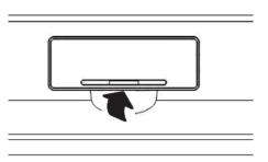
2. Insert the two pieces of AAA Alkaline bateries. Make sure they are installed properly.
