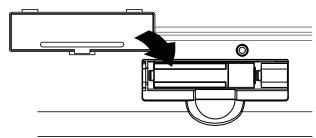
\* You don't necessarily need to install batteies if you connect the keyboard with a powerd USB port by USB cable.
