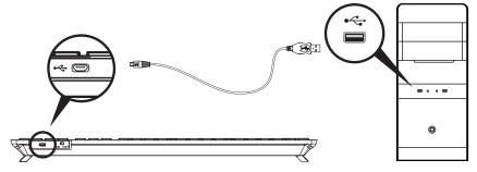
2. Select "USB" key to associate with device.\* The indicators above the USB keys will be ON.
