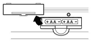
2. Insert two AA alkaline batteries and make sure the batteries are installed properly.
