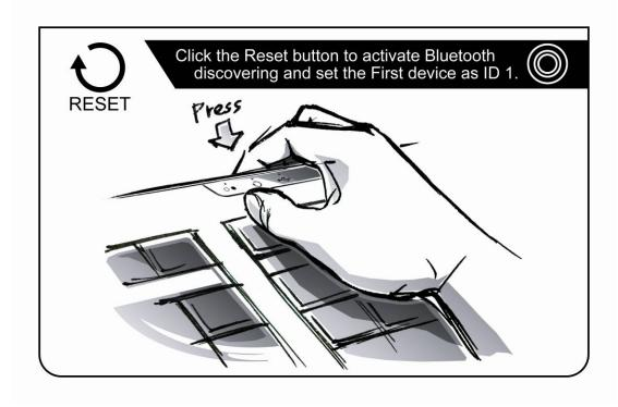
Press the Reset until the LED is flashing fast.
