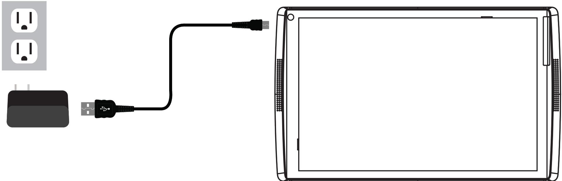
Connect the power adapter to a wall outlet, then to the Tablet as shown. It is recommended to fully charge the battery before first use. A battery status indicator appears in the lower left corner. Tap the battery icon to view percentage of remaining power.
