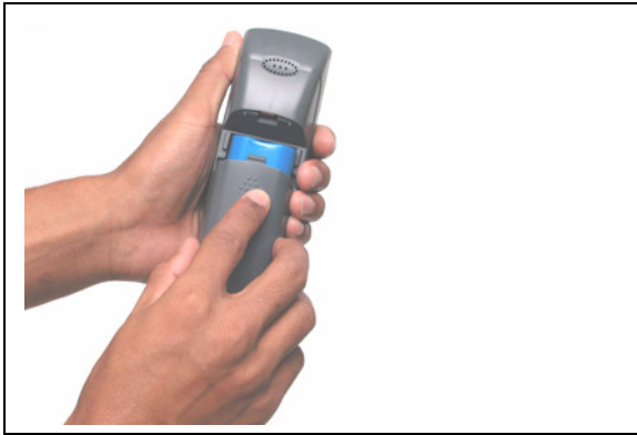
Figure 3-3 Removing the Rear Cover from the WIP2
