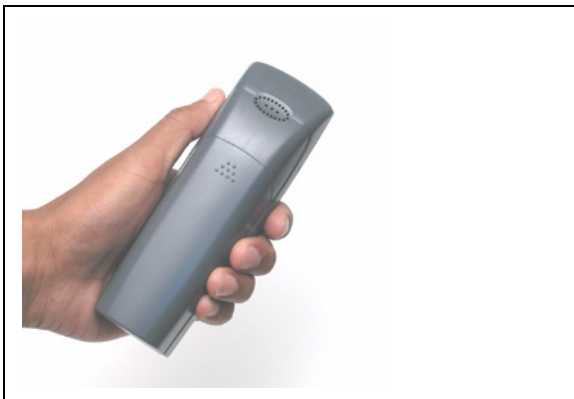
Figure 3-2 Grasping the WIP2 to remove the rear cover
