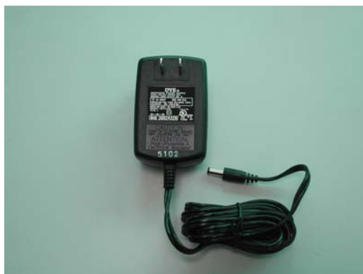
Figure 2-15 Switching Power Adaptor
