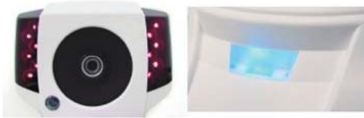
Red IR LEDs (Left), Blue Status LED (Right)
