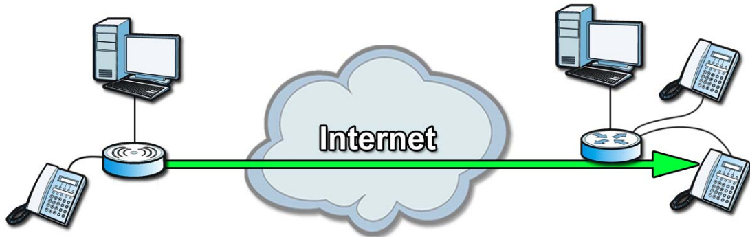
Figure 2 MAX-207HW2R's VoIP Features - Peer-to-Peer Calls
