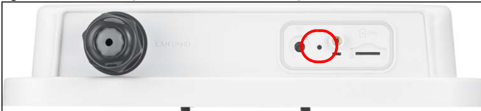
Figure 7 Reset Button (LTE7461-M602 / LTE7480-S905)
