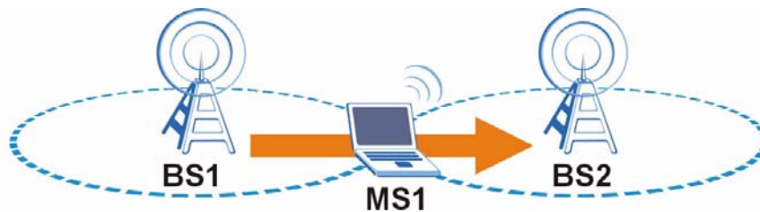
Figure 37 WiMax: Mobile Station
