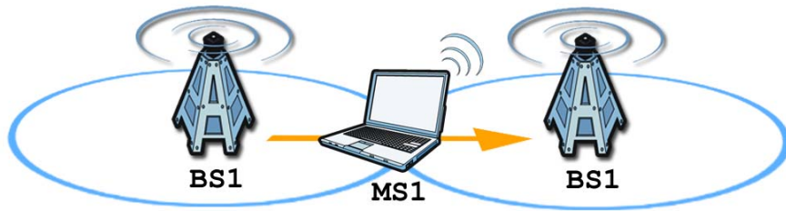
Figure 27 WiMax: Mobile Station
