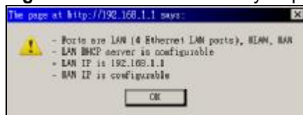
Figure 111 Maintenance > Sys Op Mode > General: Router
