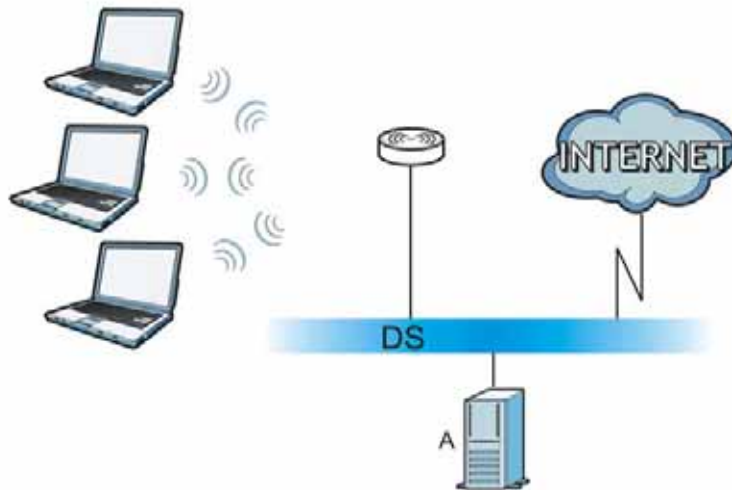
Figure 122 WPA(2) with RADIUS Application Example
