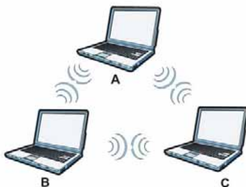
Figure 118 Peer-to-Peer Communication in an Ad-hoc Network
