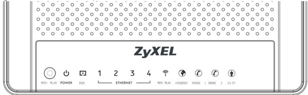
Figure 5 LEDs on the Top Panel
