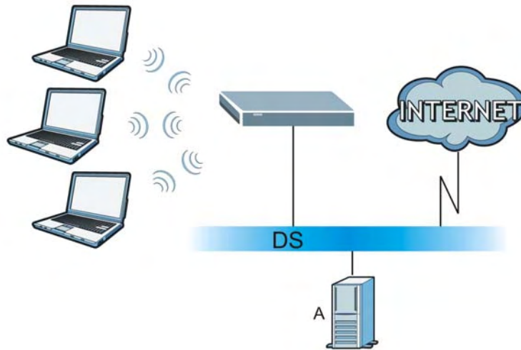
Figure 160 WPA(2) with RADIUS Application Example
