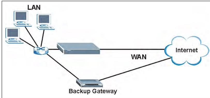
The following network topology allows you to avoid triangle route security issues when the backup gateway is connected to the LAN. Use IP alias to configure the LAN into two or three logical networks with the Prestige itself as the gateway for each LAN network. Put the protected LAN in one subnet (Subnet 1 in the following figure) and the backup gateway in another subnet (Subnet 2). Configure filters that allow packets from the protected LAN (Subnet 1) to the backup gateway (Subnet 2).
