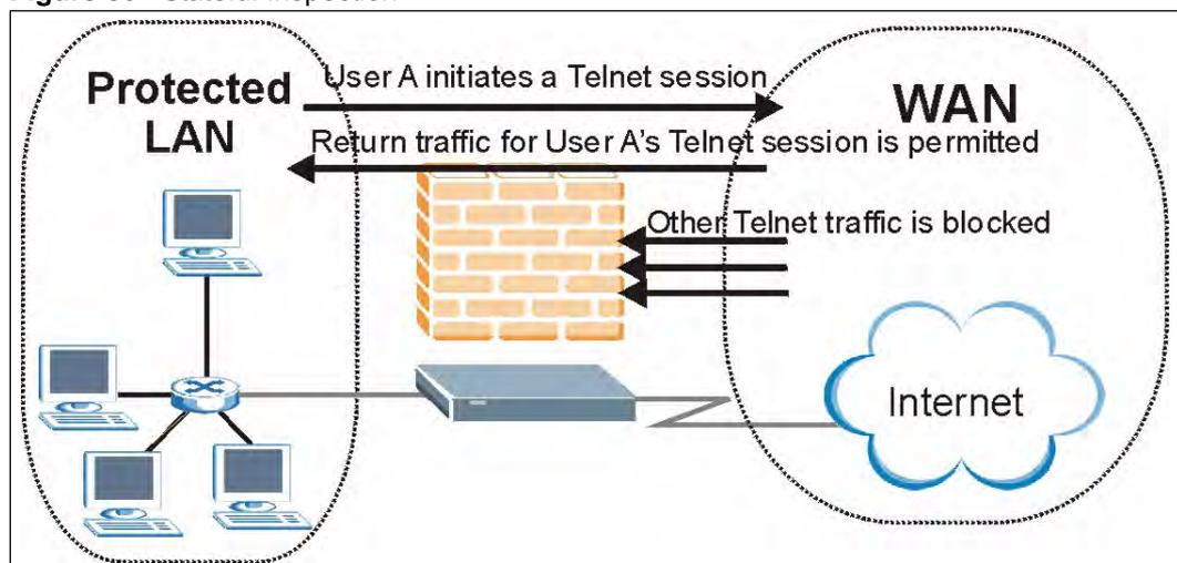
The previous figure shows the Prestige's default firewall rules in action as well as demonstrates how stateful inspection works. User A can initiate a Telnet session from within the LAN and responses to this request are allowed. However other Telnet traffic initiated from the WAN is blocked.
