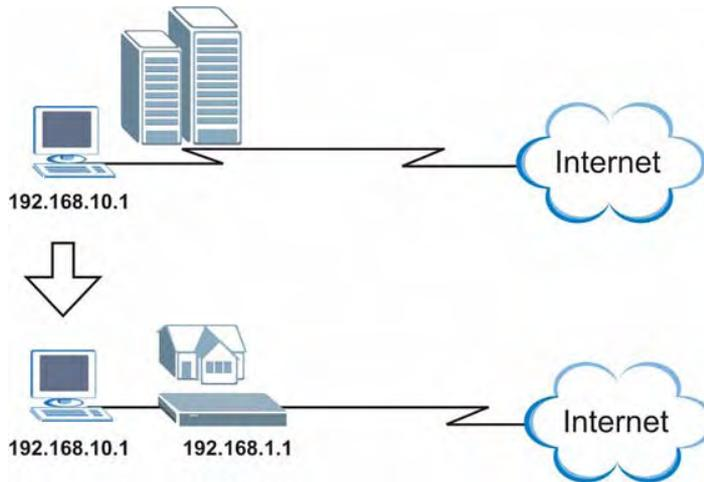
The Any IP feature does not apply to a computer using either a dynamic IP address or a static IP address that is in the same subnet as the Prestige's IP address.
