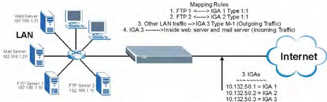
In this case you need to configure Address Mapping Set 1 from **Menu 15.1 - Address Mapping Sets**. Therefore you must choose the **Full Feature** option from the **Network Address Translation** field (in menu 4 or menu 11.3) in [Figure 156 on page 265](#).
