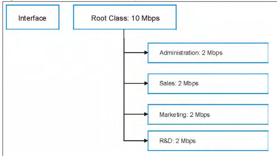
The following figure shows the bandwidth usage with the maximize bandwidth usage option enabled. The Prestige divides up the unbudgeted 2 Mbps among the classes that require more bandwidth. If the administration department only uses 1 Mbps of the budgeted 2 Mbps, the Prestige also divides the remaining 1 Mbps among the classes that require more bandwidth. Therefore, the Prestige divides a total of 3 Mbps total of unbudgeted and unused bandwidth among the classes that require more bandwidth.
