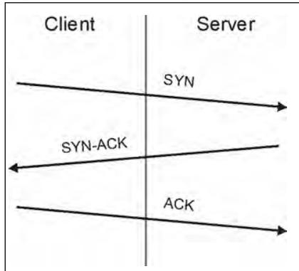
Under normal circumstances, the application that initiates a session sends a SYN (synchronize) packet to the receiving server. The receiver sends back an ACK (acknowledgment) packet and its own SYN, and then the initiator responds with an ACK (acknowledgment). After this handshake, a connection is established.
