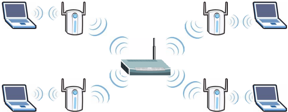
Figure 29 Connecting Wireless Networks Using WDS
