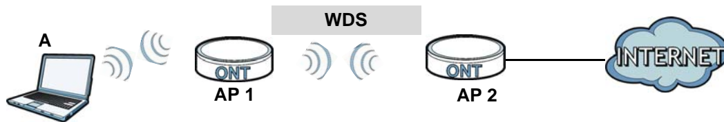
Figure 32 WDS Link Example
