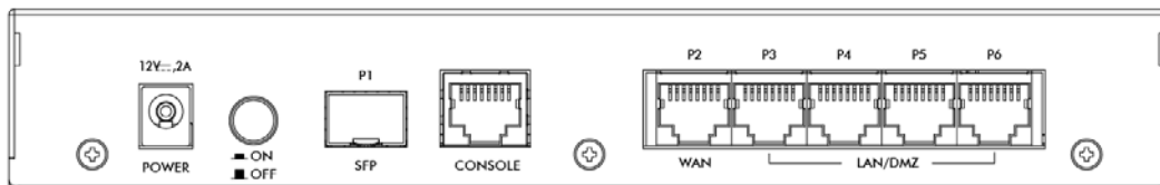
Figure 34 USG20W-VPN Rear Panel
