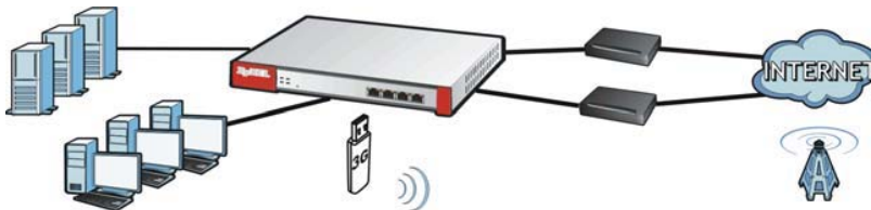
Figure 6 Applications: Multiple WAN Interfaces
