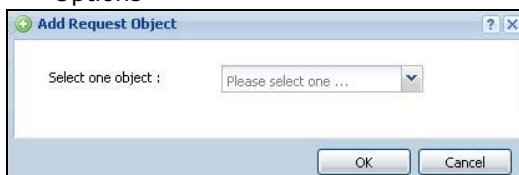
Figure 123 Configuration &gt; Network &gt; Interface &gt; Ethernet &gt; Edit &gt; Add DHCPv6 Request/Lease Options
