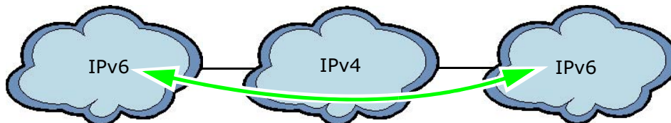
Figure 131 IPv6 over IPv4 Network
