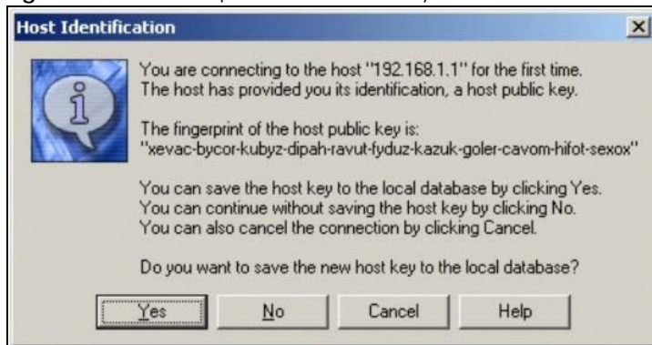
Figure 87 SSH Example 1: Store Host Key
