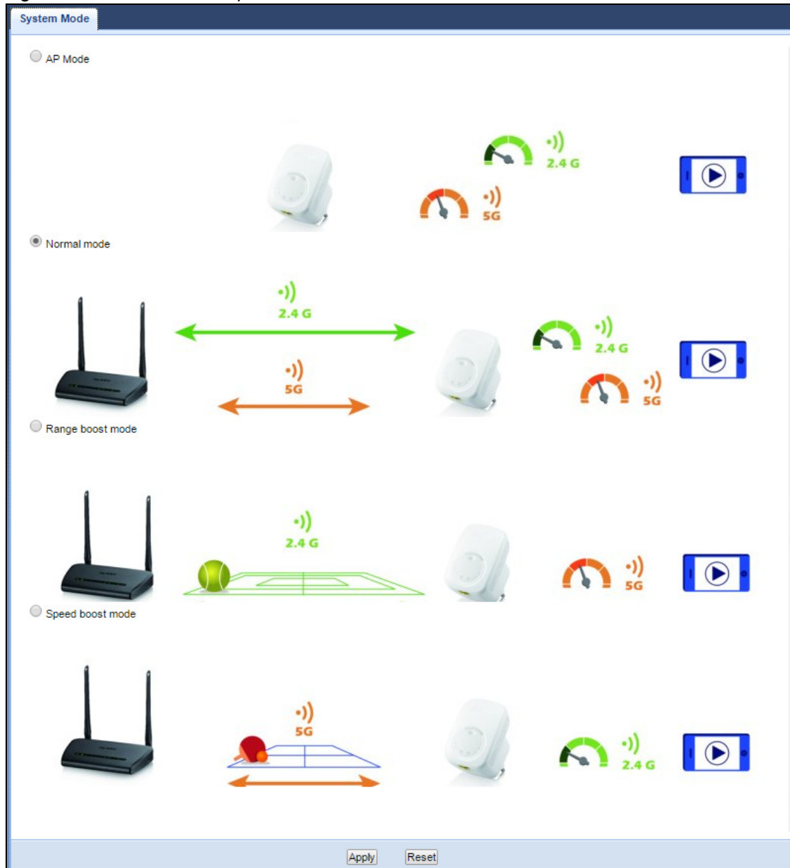
Figure 56 Maintenance > System Mode
