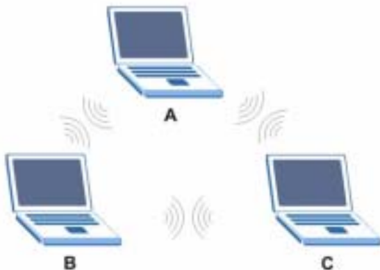
Figure 202 Peer-to-Peer Communication in an Ad-hoc Network
