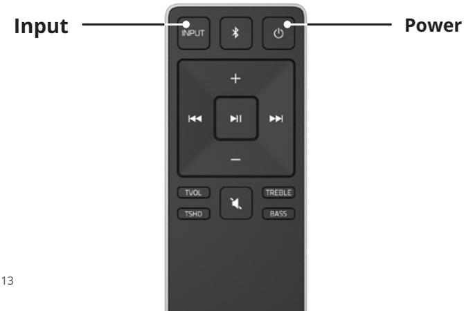
\* Auto detect function only occurs once when Sound Stand is first powered on. To enable this feature again, you must do a Factory Reset or **Press and hold** the **INPUT** button on the remote control for 5 seconds to enable the auto input detect function.
